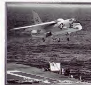
▲ Raised wing The Crusader has a variable-incidence wing, which reduces speed when the aircraft lands.
